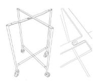
Open the frame and stand in an upright position. Use the hardware provided to secure the frame together.
